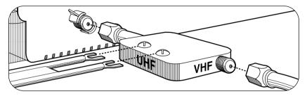
If your antenna system has two sets of twin 300-ohm leads, you must obtain a combiner (available at your local electronics store). Place one set of twin leads underneath the screws on the combiner and tighten the screws. Do the same with the other set of twin leads. Press the cable from the combiner onto antenna terminal on the back of your TV.
